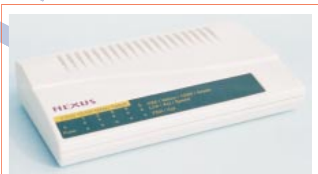
As you can see, a five-port switch looks very similar to a five-port hub. However it has the capability to give much speedier network operation. This Nexus 10/100BaseT unit is sold by Electus dealers as the YN-8082.
