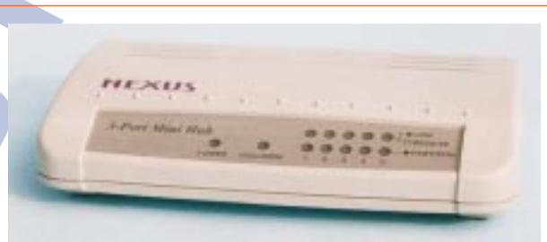
This very compact 10BaseT five-port hub is very suitable for small networks. One of its five ports can be configured as an 'uplink' port, with the connections internally crossed over. Power comes from a small 'plug pack'. The Nexus unit shown is sold by Electus dealers as YN-8070.
