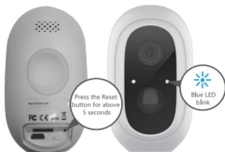
**Step 4:** Press and hold the reset button for up to 5 seconds, then release the button to reset the camera. The LED light will blink quickly.
